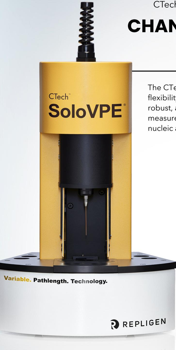
The CTech™ SoloVPE® System leverages the power and flexibility of variable pathlength technology to create a rapid, robust, and repeatable, non-disruptive concentration measurement method for proteins, plasmid DNA, and nucleic acid modalities, with results in minutes, not hours.
