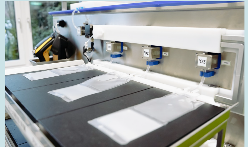
Figure 4. RoSS.FILL filling unit.
