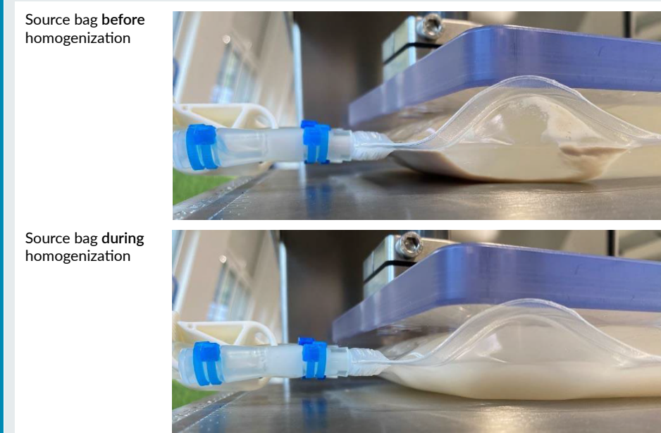
Figure 1. Homogenization of Saccharomyces cerevisiae yeast cells with the automated RoSS.PADL system.
