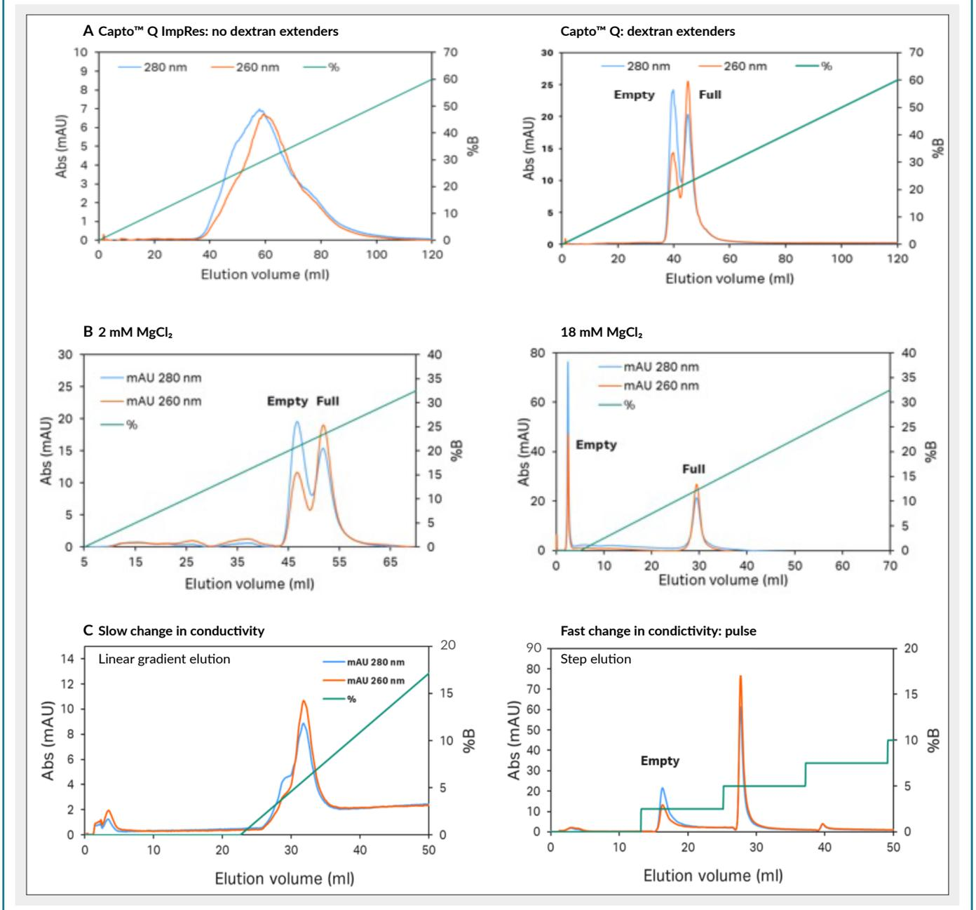
At higher concentrations of magnesium chloride, empty capsids elute before the salt gradient application and the full capsids in the gradient, resulting in a baseline separation.
