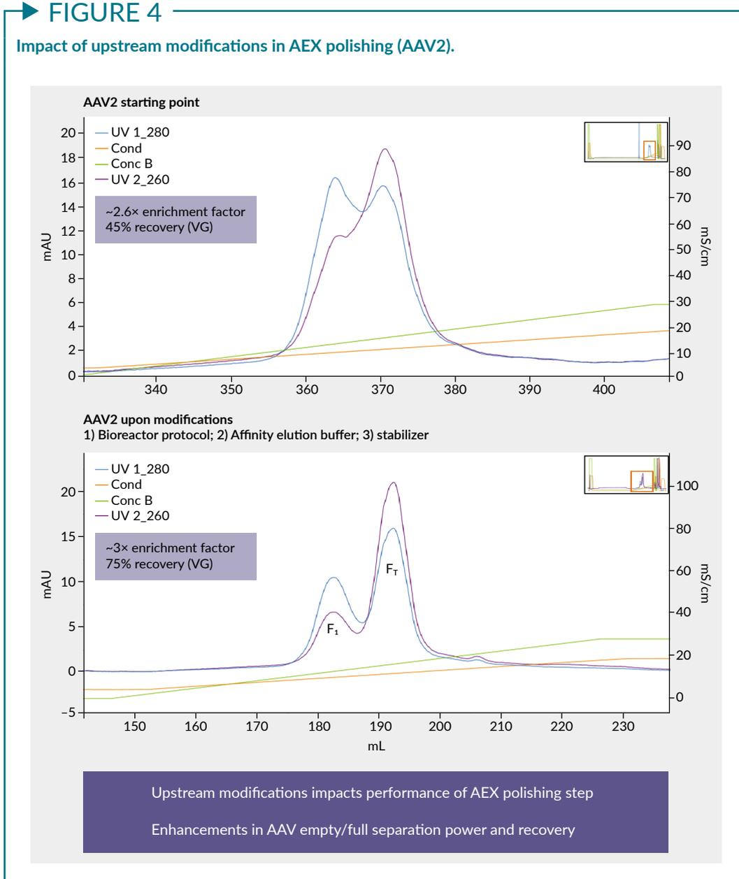
increasing pH values leading to a significant decrease in AAV recovery. For the alternative resin, this effect was slightly negative. The results demonstrated that approximately 75% recovery was achievable with AAVX resin, a considerable improvement on the initial 53% recovery.
