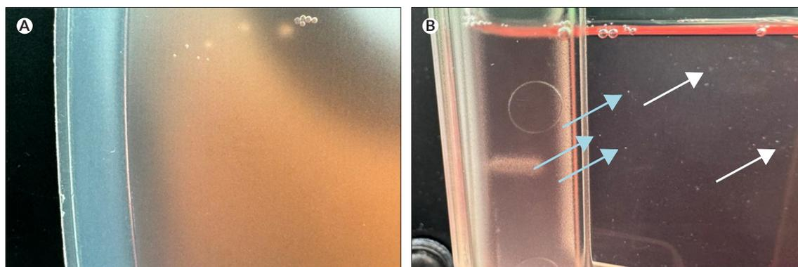
Images were taken at identical distances under identical 2x magnification. Both containers were filled with non-filtered cell culture media. Floating aggregates or fibers (white arrows), and microbubbles (blue arrows) were detectable in the CryoCase but were undetectable in the bioprocessing container.
