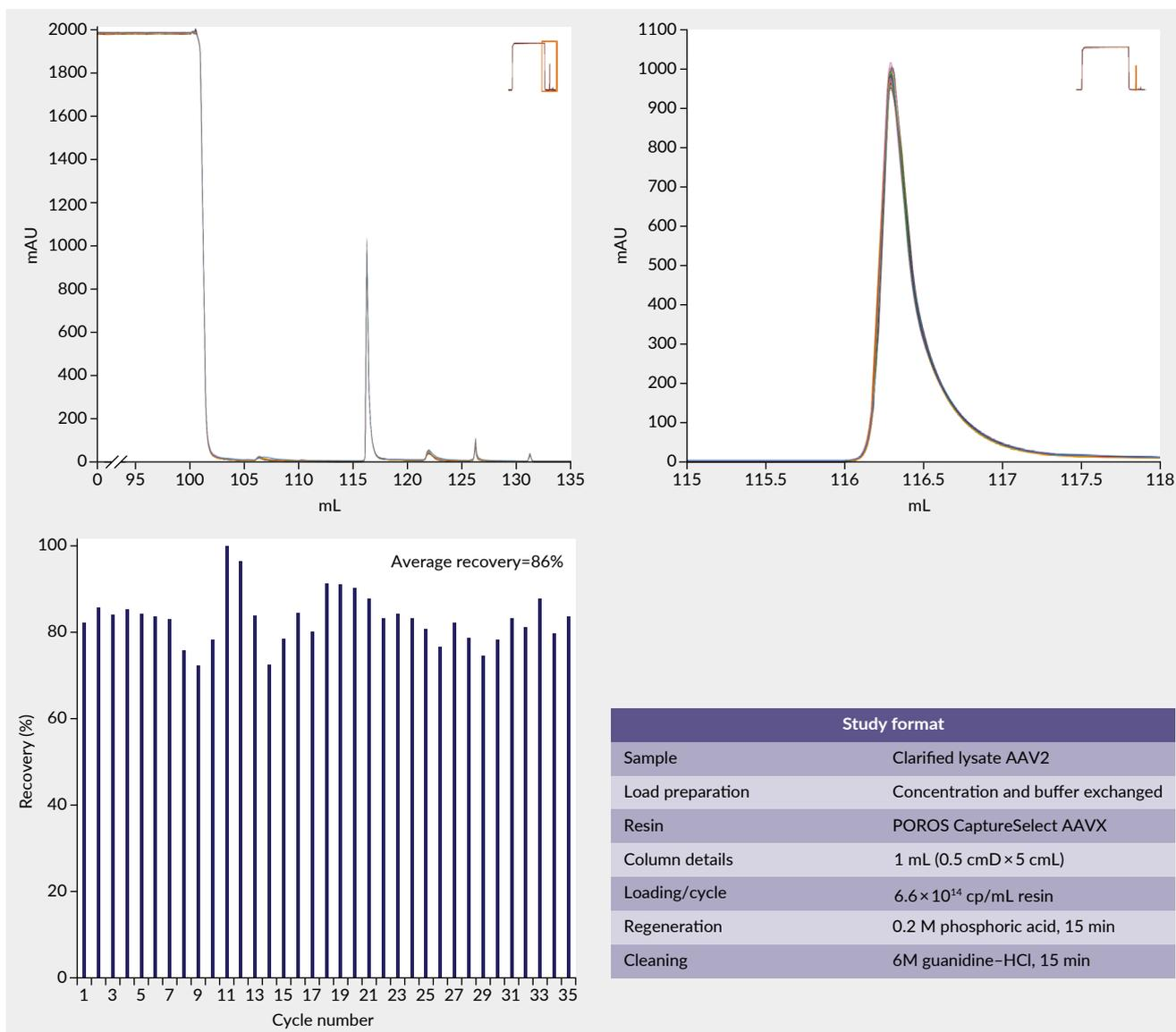
$>1 \times 10^{15}$  capsids/mL resin at residence times  $\geq 30$  sec for AAV2 can be achieved with POROS CaptureSelect AAVX. Productivity is maximized at load residence times  $\leq 30$  sec depending on titer, but hardware and/or system considerations limit operation closer to 1 min. It is also possible to determine a window of operation based on the maximum back pressure that can be accepted. Process calculations suggest that for large bioreactor volumes (e.g., 2000 L) and high titers
