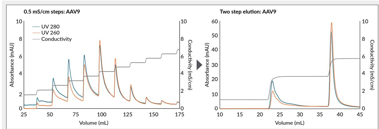
The changes of the UV260:UV280 ratio inform selection of the conductivity for elution of AAV9 empty capsids in the final two-step protocol using Mustang Q.
