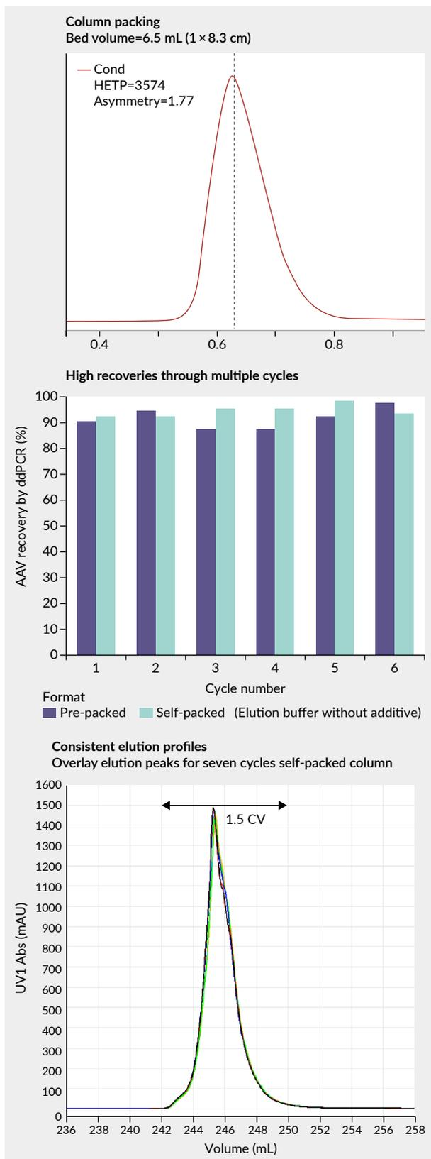
self-packed and pre-packed resins, and performance remained consistent over 7 cycles, demonstrating that minimal protocol adaptations were needed when transitioning from AAV2 to AAV8.
