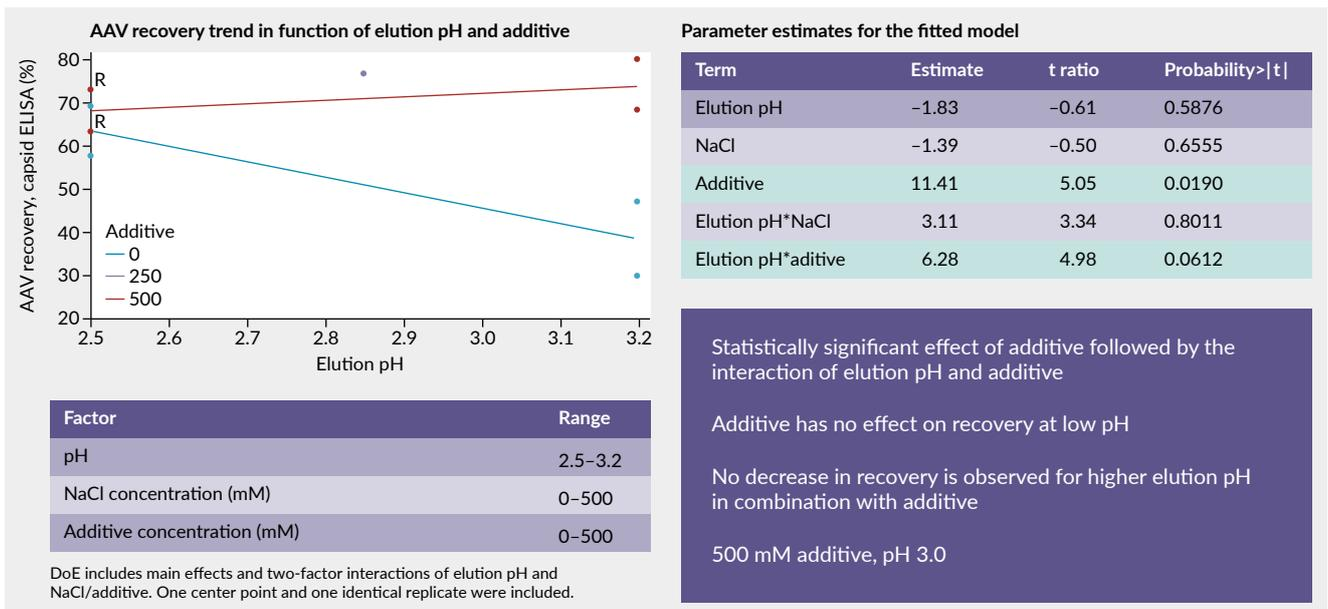
column type, loading density, and elution pH on AAV recovery. Results shown in **Figure 2** show that the effect of loading density was not significant. Interestingly, the effect of elution pH depends on the column resin used. For AAX resin, this was highly negative, with
