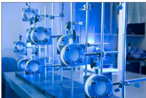
Membrane viral penetration test set-up.
